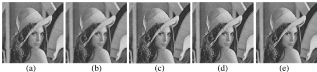
Figure 1 - Visual comparisons of denoising results on Lena image corrupted by additive white Gaussian noise with standard deviation 30: a. Wiener filtering; b. Bilateral filtering; c. PCA method; d. Wavelet transform domain method; e. BM3D [22]
