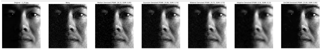
(a) 1. Original image; 2. Noisy image; 3. Median Denoised; 4. Gaussian Denoised; 5. Bilateral Denoised; 6. NLM Denoised; 7. DnCNN Denoised
