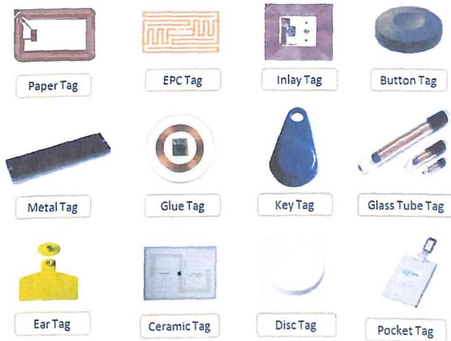
Figure 4.2: RFID Passive tag types
