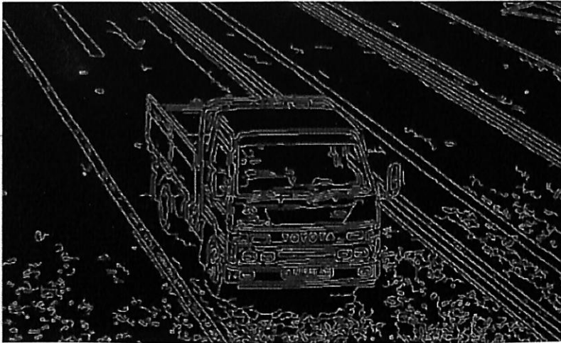
Figure 3.5: Filtering using the Canny edge detector.
