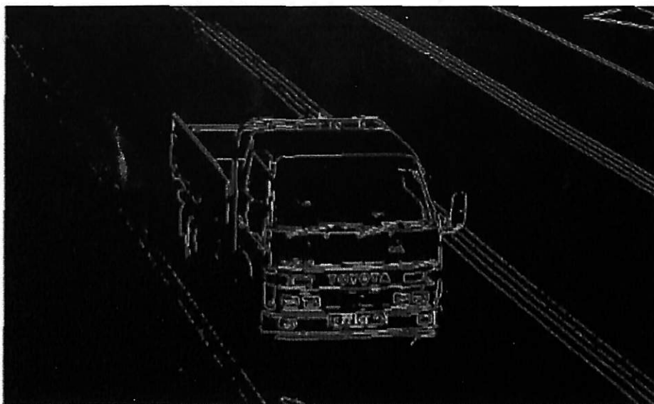
Figure 3.7: Filtering using the Pruet operator.
