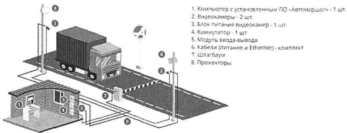
Figure 2.1: Typical composition of equipment for single-track control
