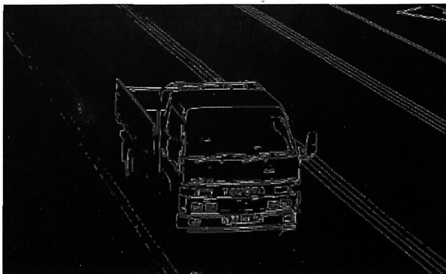
Figure 3.4: Filtering using the Sobel operator.
