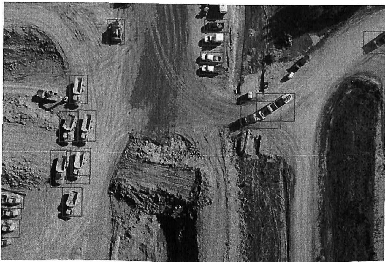
Figure 2.17: The result of the DetectNet neural network is shown, which is trained to detect vehicles in aerial images.
