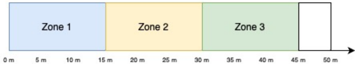
Figure 3.2 – Modeling a Zone-Based Acoustic Sensor System for UAV Distance Prediction
