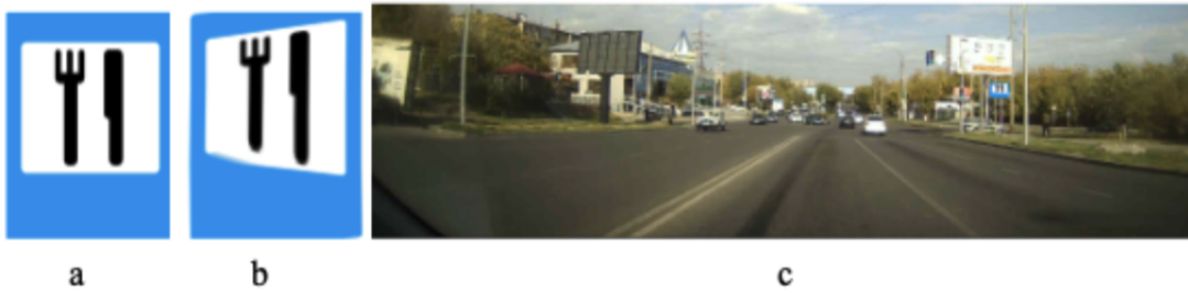
Figure 4.2 – Augmentation pipeline in an example of food point sign: (a) initial sign, (b) geometric augmented sign, (c) background integrated sign
